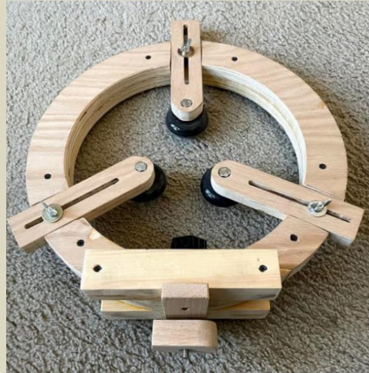
Steve Halliday: Home-made steady rest. The circle is made from 3/4" plywood with other portions made from red oak. The circle is approximately 12" in diameter. The 3 supports with roller blade wheels are 6 1/2" long.
