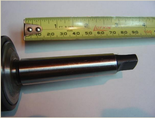
Measuring the Morse taper
