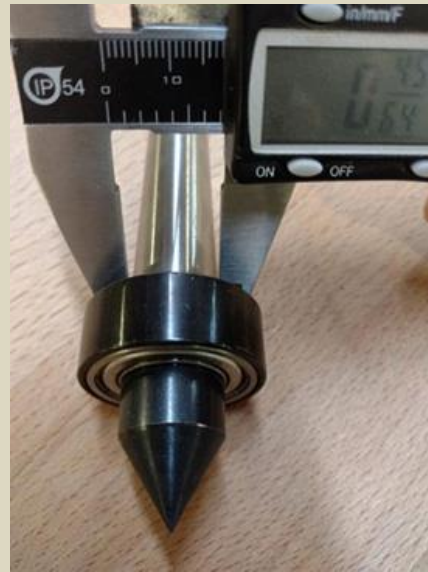
Measuring the Morse taper
