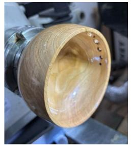
A coat of final finish is now added to the bowl. I chose Waterlox Original. This is a catalyzed tung oil finish and is food safe when dry. I wanted a finish that the user did not have to worry about. I put two coats on the bowl.
