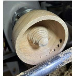
Bowl is hollowed out being careful to leave enough supporting mass in the bowl until the top section is to the correct thickness. I chose about ¼ inch.
