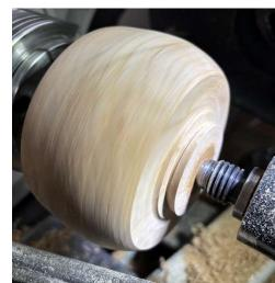
After turning it to rough shape I made a tenon.
