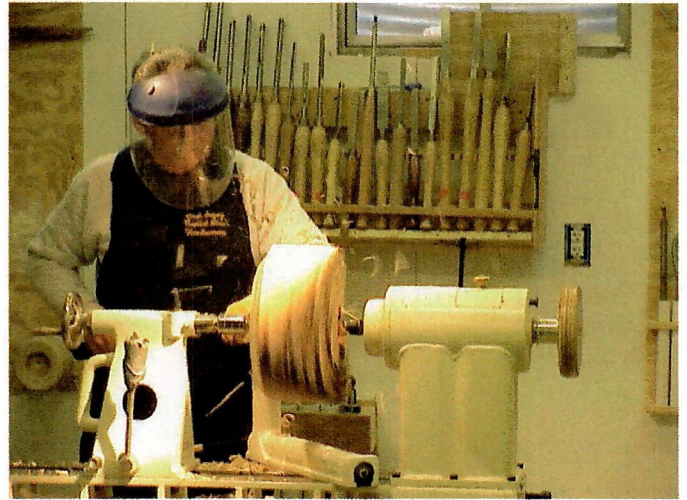
C.A. Savoy practices what he preaches when it comes to safety procedures. Here, he begins to rough out a bowl and shape the base for the tenon.
