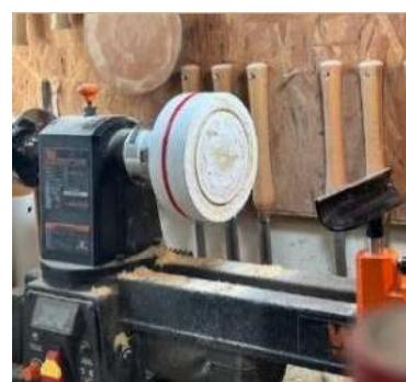
*Most support blocks are relatively thick. The thickness provides enough mass to reduce vibration and chatter while you are cutting.*
