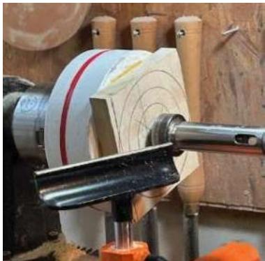
*The work piece is mounted to the support block so that the largest cutting diameter is fully supported. The work piece is hot glued to the support block and (if needed) I use the tail stock for additional support.*
