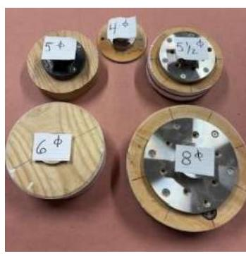
*I made several support blocks of various diameters, 4, 5, 5 1/2, 6 and 8 inch. Some are screwed to the faceplate. Others have a tenon to fit my chucks.*
