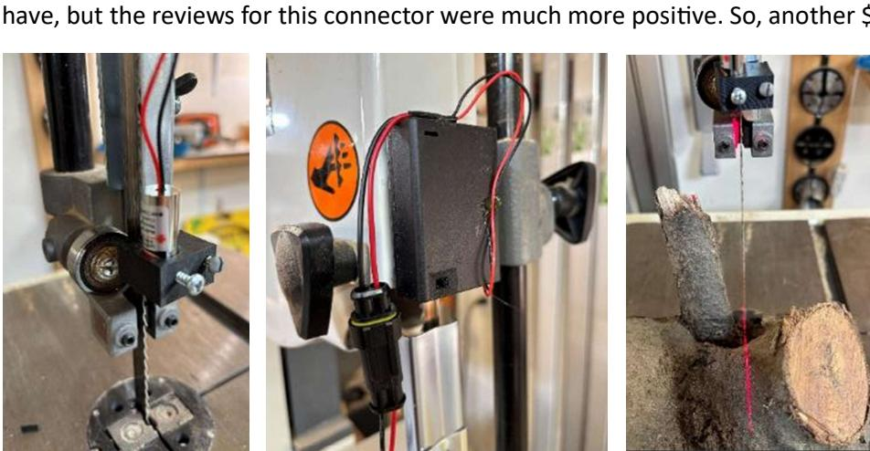
The final unit is great. For less than \$30, I have a laser guide that will help me as I start on some of the new turning projects I have in mind.
