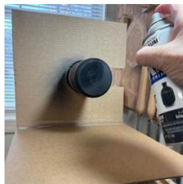
Step 2: Cut a slot in the cardboard large enough to slip onto the spindle body BEHIND your chuck. Location is important for a secure fit. So remember, measure carefully. I used a pencil, ruler and square to layout my slot.
